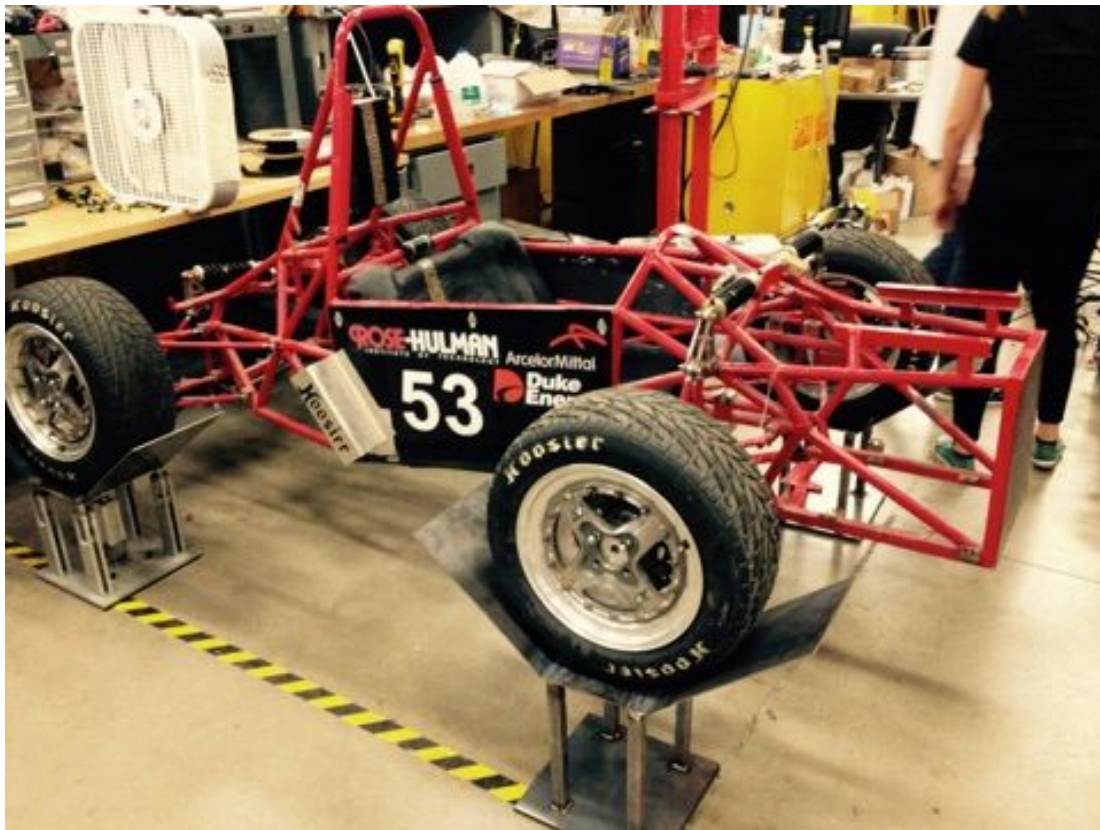
Figure 6 - Frame Used for Mock Up on Test Stands
